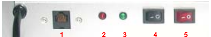
1. LAN 2. HD LED 3. POWER LED 4. Rest 5. POWER
